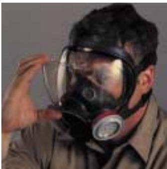
For nuclear personnel, the lens shield provides an additional level of eye protection and increased beta-radiation protection — increasing combined lens density thickness to 500 mg/cm<sup>2</sup>.
